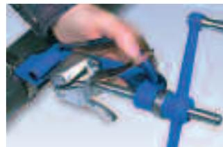
7. To set the lock and cut off band, roll tool nose over buckle, relieving a slight amount of tension by backing off tension handle during this fold over operation. Failure to back off tension handle throughout the entire course of roll over may result in breaking band. On the other hand, releasing too much tension may result in a loose clamp.
