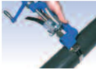
6. Place band in open slot of tool nose and gripper block. Move into slot as far as possible to prevent buckle from sliding into tool nose. With thumb on band gripper lever, apply tension by turning handle of tool. After tension is created, it is no longer necessary to hold the band gripper lever as it locks itself under tension. When band stops moving through buckle, maximum tension has been applied. Stop turning handle.
